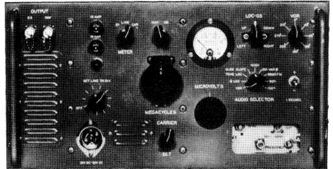
479T-2 ALL CHANNEL VOR-ILS SIGNAL GENERATOR — A portable test set for ramp testing of navigation and ILS receivers. May be used inside or outside the plane for an over-all check on the installation from receiving antenna to indicating instruments. Complete coverage of all channels from 108.0 through 135.9 and 329.3 through 335.0 mc. RF level can be varied from 4 to 200,000 microvolts. Signals include: VOR, LOC, glideslope, 1000 cps audio tone. Size: 19" W, 18" H, 10½" D.
