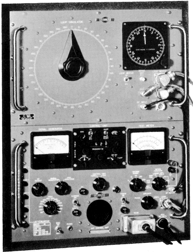
477U-1, 477V-1 ADF TEST SET — Provides complete test and simulator signals for the DF-201 ADF. The 477U-1 ADF Loop Simulator generates a calibrated RF field and excites a contained loop antenna. Receiver bearing indications are displayed on the front panel. The 477V-1 tests antenna, loop, ADF aural and ADF bearing sensitivity, dial calibration, bearing speed, AVC and gain control characteristics, and makes test point measurements on individual modules. Mounting: Rack or carrying case.
