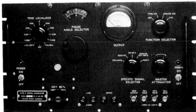
479S-3 VOR AUDIO SIGNAL GENERATOR — Used for precision testing and calibration of VOR receivers. It provides all output signals required for VOR, tone localizer and
